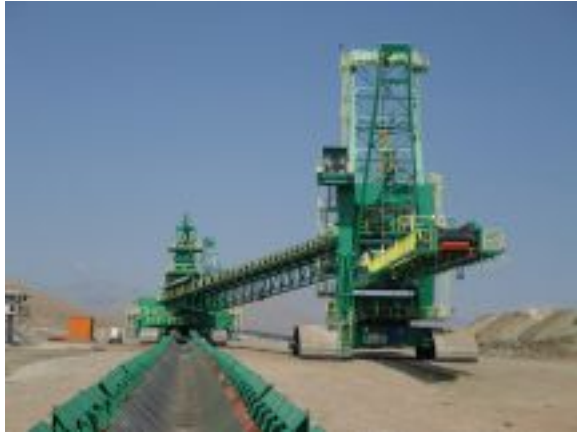
Spreader ARS 1800, detail: belt conveyor View image
