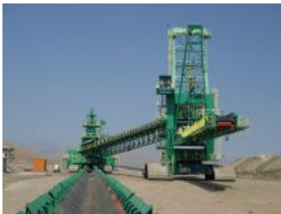
Spreader ARS 1800, detail: belt conveyor
