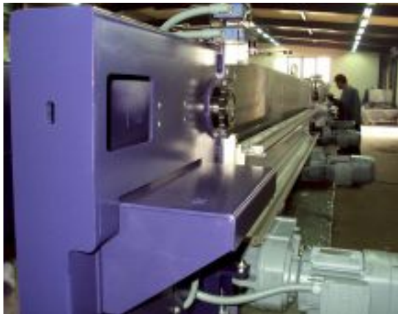
Mounting of the sheet handling system View image
