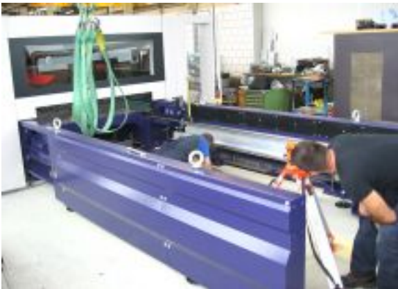
Mounting of the laser cutting machine assembly View image
