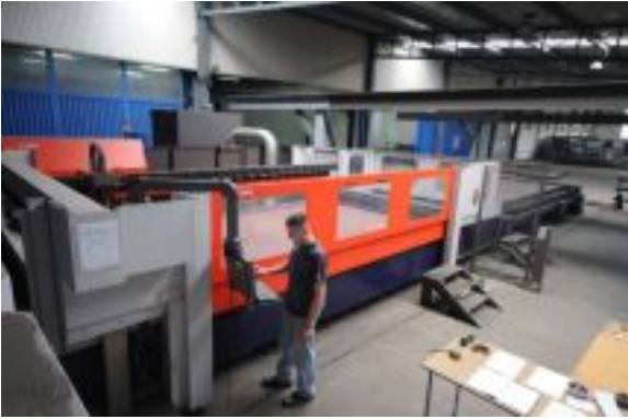
CNC laser cutting machine (Bystronic Laser AG), laser strength 6000 W
